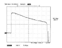
Shown here is a typical clamp waveform of the Model 160.
