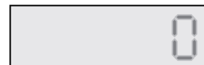
Fig. 5a: Upon startup for the PT250 and -EC models, counter should read zero. If a non-zero is displayed, the counter can be reset by following Step 6. If the counter is blank, contact MCG Support at 1-800-851-1508.
